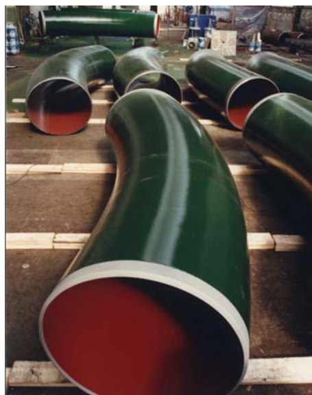
Figure 10: Iamsub coated 7D-bends with epoxy resin lining inside, size 48" in Grade L 555 MB
