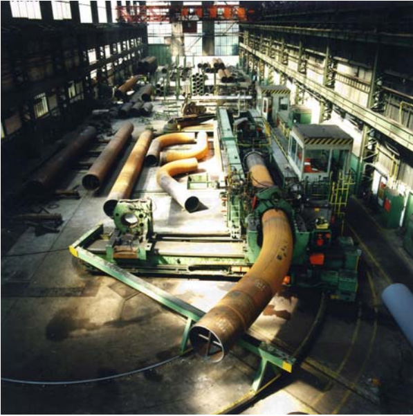
Figure 8: Hot induction bending of 48" line pipe at Mannesmann Bending Plant
